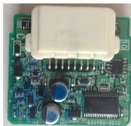
Immobilizer control module Tokai Rika. It is with EEPROM 93C66. Dump is ENCRYPTED!
