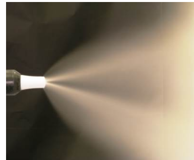
too much electrode rinsing air
